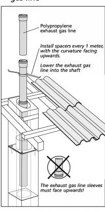
5 Installing the roof duct and adjustable roof tile
