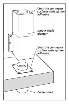
3 Installing the shaft in the roof area
