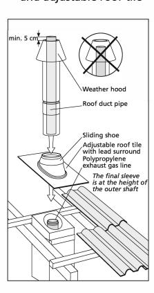
6 Installing the connector T-piece
